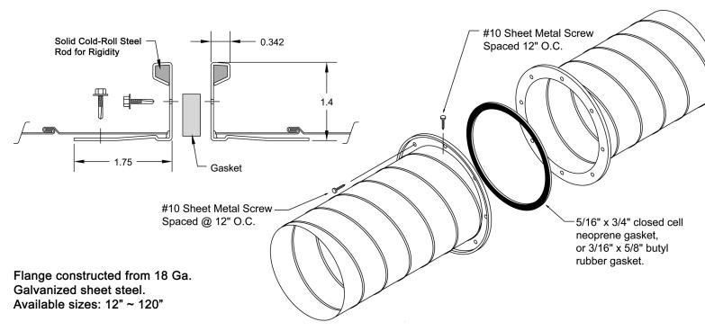
The use of the DuraFlange connecting system, installed and sealed per manufacturer's recommendations, is suitable for use on all systems across a range of internal duct pressure classes; from positive 10" S.P.W.G. to negative 6" S.P.W.G.
